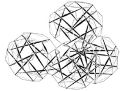
Fig.19.1 D.G. Emmerich's monograph Tensile and self-tensioning structures, showing a tensegrity structure composed of truncated octahedrons assembled by derotating the square faces forming octagons.
