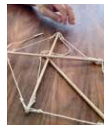
Fig. 10.5 Still no Tensegrity due to one unconnected tendon.
