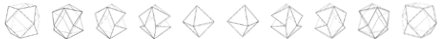
Fig.16.4, A TS-Icosahedron with solid faces and its corresponding transformation from expansion to compression and back to expansion.
